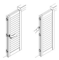
Do not pull the panel facing you to close. Bi-fold  $180^{\text{TM}}$  is not designed to move this way.
