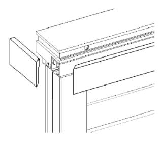
On wood fascias, take off the sticker backing of the styrofoam tape on the back of the fascia. Position the fascia along the header groove evenly and press inward to secure.
