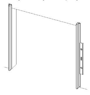
Secure the light blocks to the wall with the provided screws as shown below
