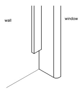
Take note that that the light block runs all the way to the floor. Therefore, please remove obstructions such as baseboard sections or moldings that would prevent the light block from mounting straight onto the wall and the floor.
