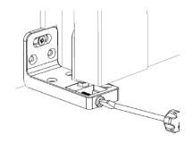
Adjust left or right by adjusting the top screw
