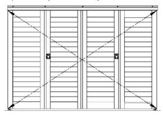
If the top needs to be adjusted left or right, use a screwdriver to tighten or loosen the screw on the top bracket as pictured
