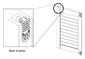
Remove the cap on the panel hanger. To remove, loosen the button screw of the cap. Then lift the cap up, and gently pull outward as shown. Put the cap aside.
