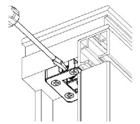
For the Bottom Pivot L Bracket, you can adjust left or right, as well as in or out. Tighten or loosen the screws as pictured
