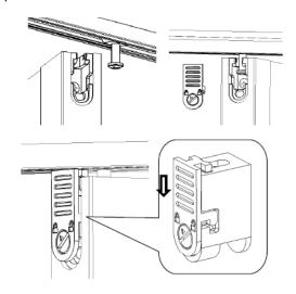
When the screw cap is fit into place, secure it by turning the dial to lock.
