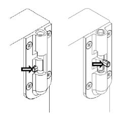
Match up the pivoting knob to the hole of the top bracket. Then disengage the pin from the middle position to the top position as shown. The pivoting knob will then automatically click into place.
