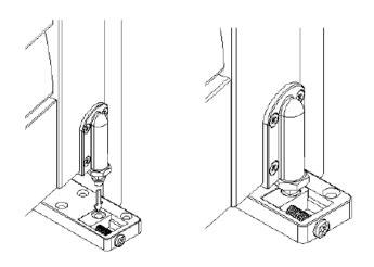
To install the top pivot, first disengage the pin to the middle position.
