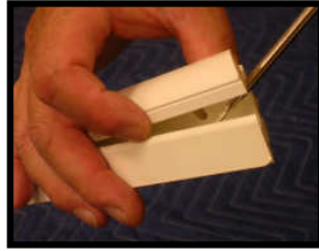
CAREFULLY lift up on the screwdriver to separate frame from filler strip.
