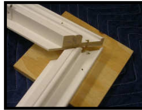
Push top frame down onto the Hoffman Key.
